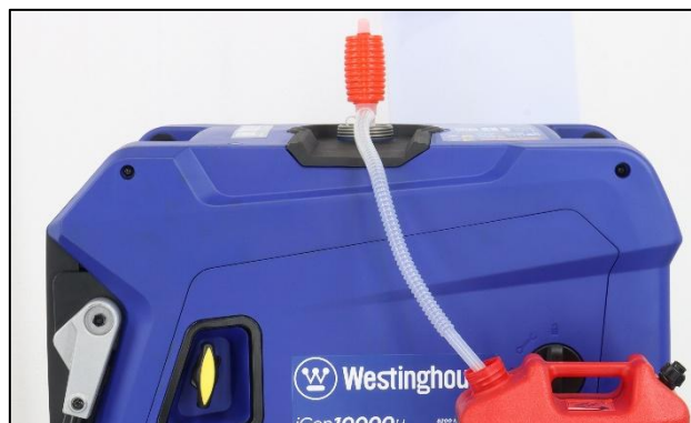
Figure 36 Drain the Fuel Tank
