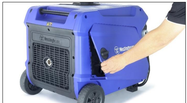
Figure 27 Remove the LHS Access Cover
