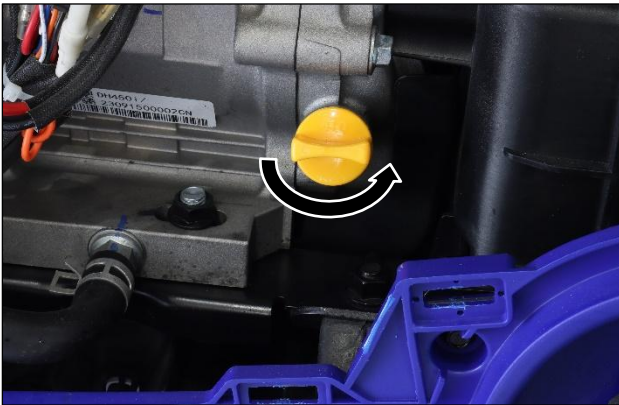
Figure 28 Remove the Oil Fill Plug
