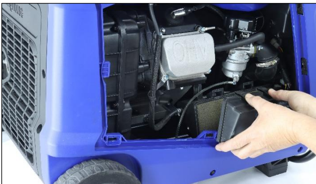
Figure 32 Remove the Air Filter Cover
