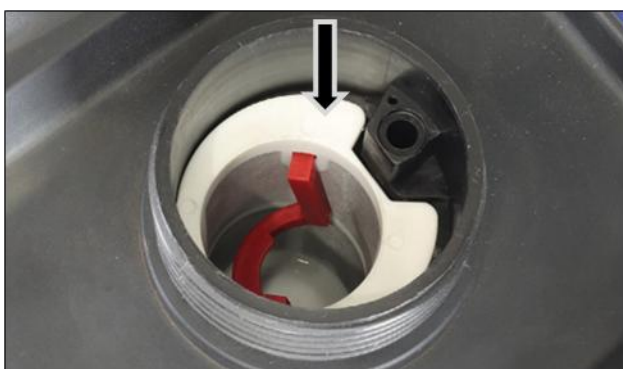
Figure 35 Install the Fuel Strainer
