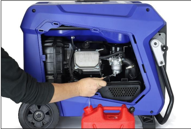
Figure 37 Drain the Carburettor
