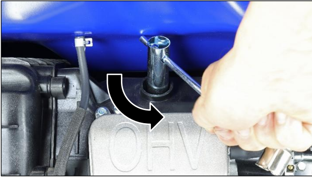
Figure 40 Remove the Spark Plug
