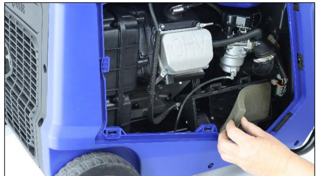
Figure 33 Remove the Air Filter Element
