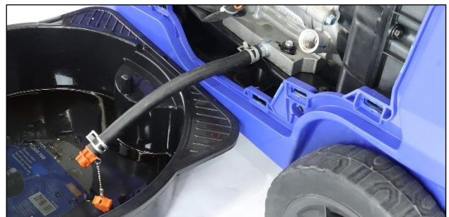
Figure 31 Drain the Engine Oil
