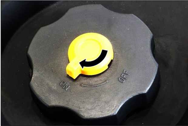
Figure 9 Fuel Cap Vent in the ON Position
