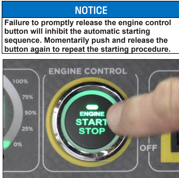
Figure 14 Press the Engine Control Button
