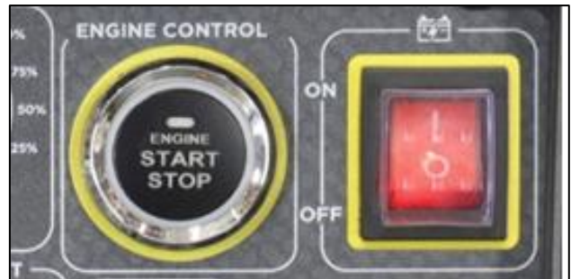
Figure 12 Battery switch in the ON Position
