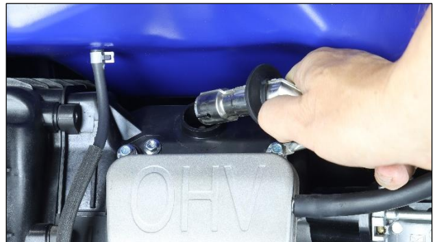
Figure 39 Remove the Spark Plug Boot
