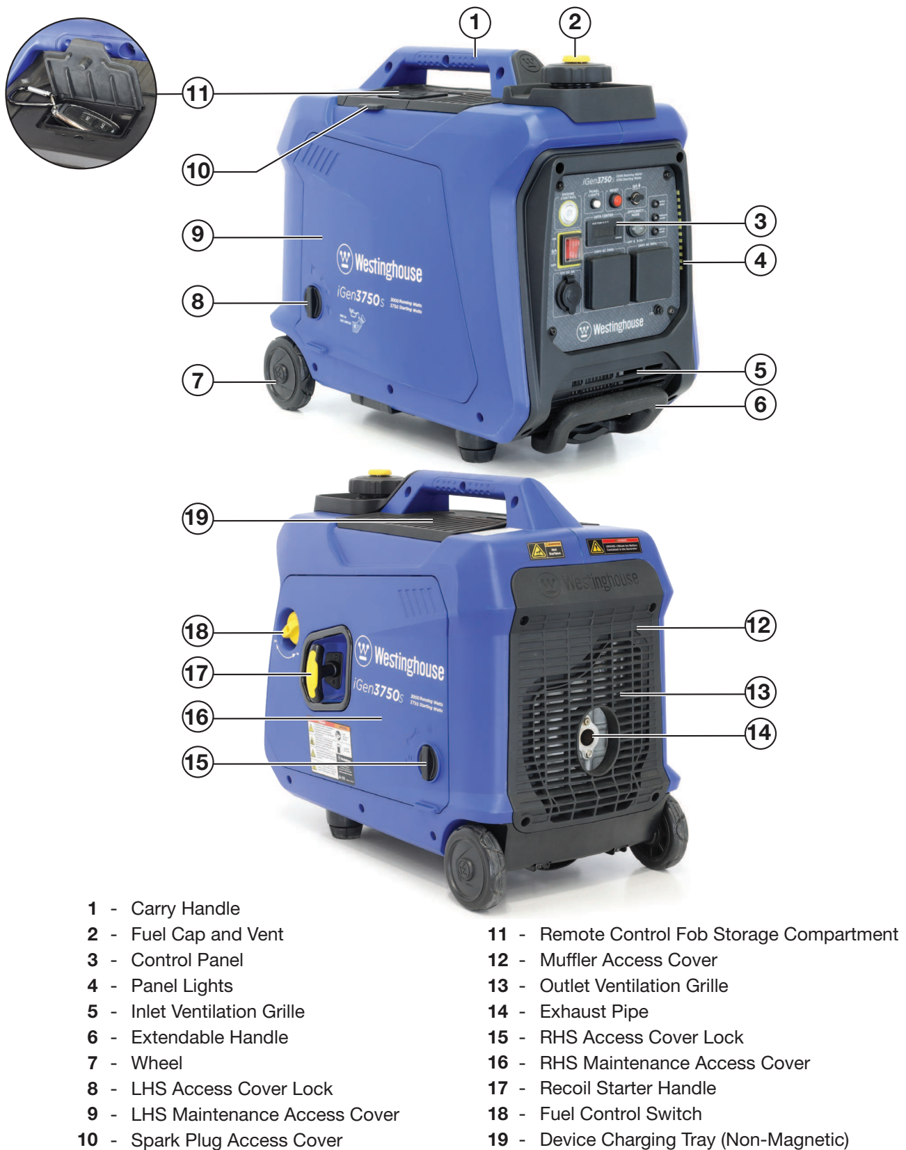
Figure 3 - iGen3750s Main Generator Components
