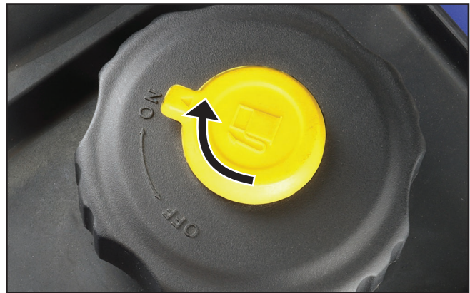
Figure 10 – Fuel Cap Vent in the ON Position
