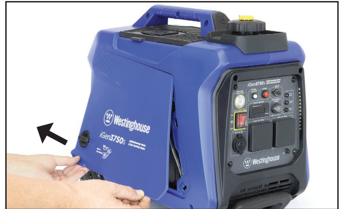
Figure 6 – Removing the LHS Maintenance Access Cover
