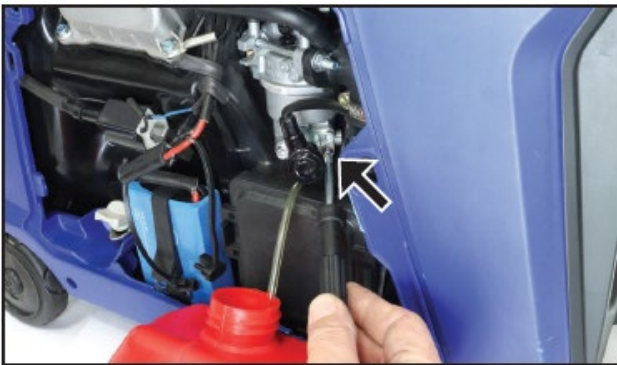
Figure 35 Drain the Carburettor
