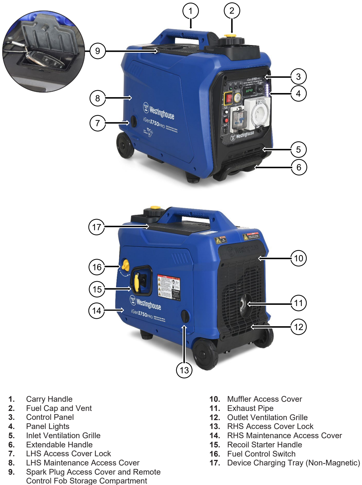
Figure 3 iGen3750PRO Main Generator Components
