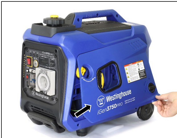
Figure 22 Remove the RHS Access Cover
