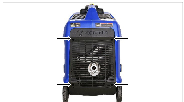
Figure 25 Remove the Muffler Access Cover
