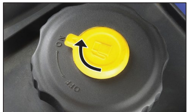
Figure 7 Fuel Cap Vent in the ON Position
