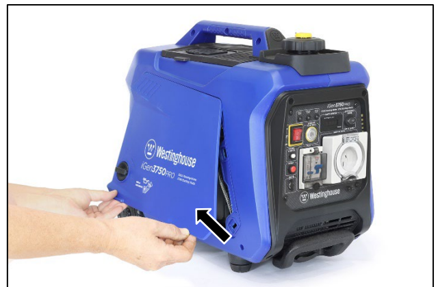
Figure 24 Remove the LHS Access Cover
