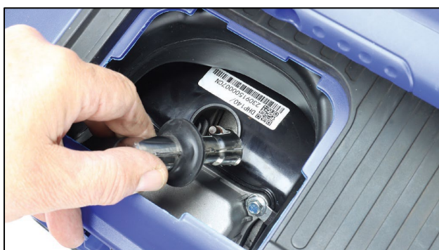
Figure 39 Remove the Spark Plug Boot
