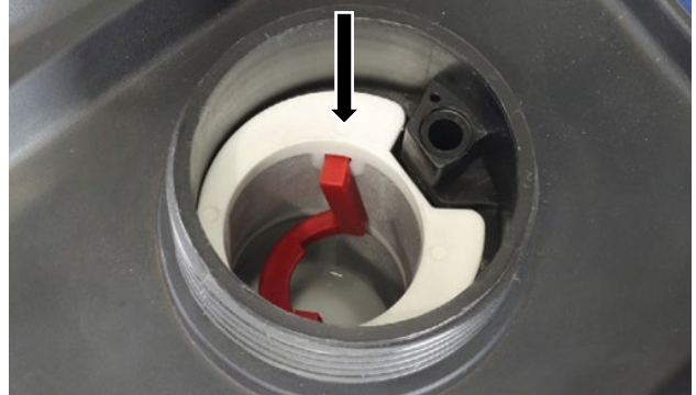
Figure 33 Install the Fuel Strainer
