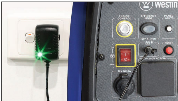
Figure 17 Connect the Battery Charger to Mains Power Supply
