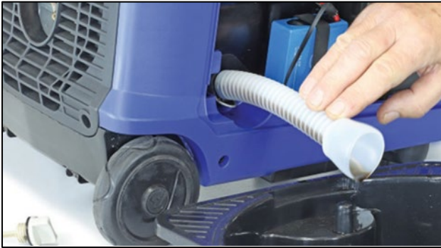
Figure 29 Draining the Engine Oil
