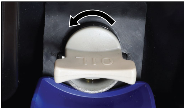
Figure 26 Remove the Oil Fill Plug
