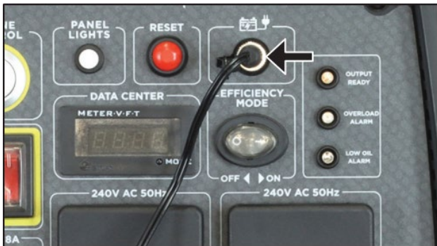
Figure 16 Connect the Battery Charger to the Generator
