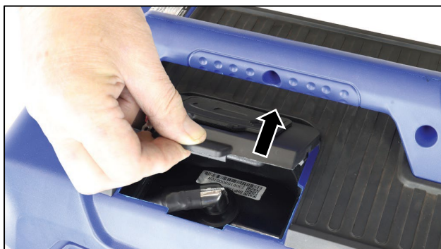
Figure 38 Remove the Spark Plug Access Cover
