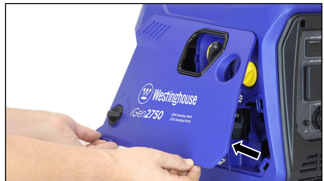
Figure 15 Remove the LHS Access Cover
