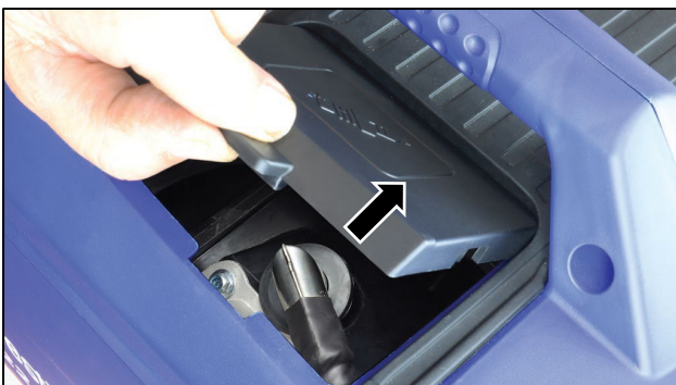
Figure 28 Remove the Spark Plug Access Cover
