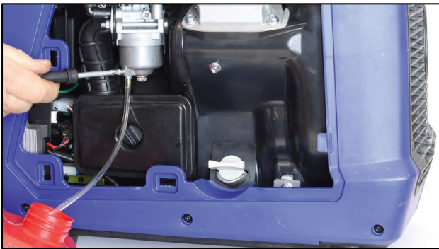
Figure 26 Drain the Carburettor
