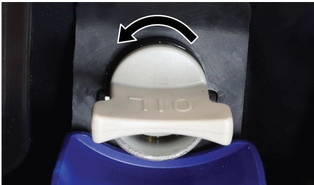
Figure 17 Remove the Oil Fill Plug
