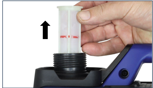
Figure 23 Remove the Fuel Strainer
