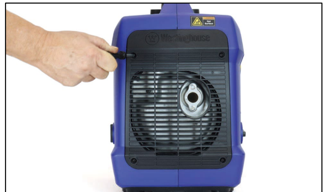
Figure 16 Remove the Muffler Access Cover
