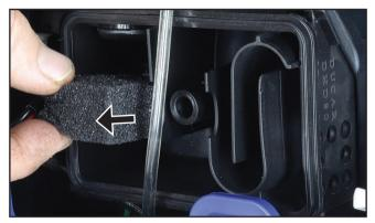
Figure 19 – Removing the Air Filter Element
