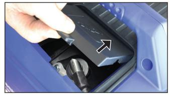
Figure 22 – Removing the Spark Plug Access Cover
