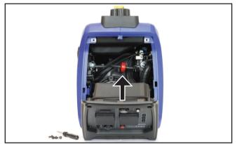
Figure 28 – Replacing the Fuel Filter
