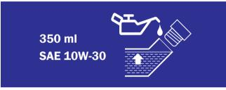
Figure 15 – Checking Oil Level
