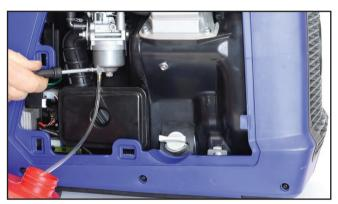
Figure 34 – Draining the Carburettor
