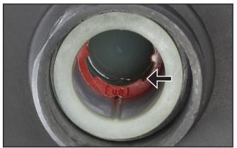
Figure 5 – Maximum Fuel Fill Level
