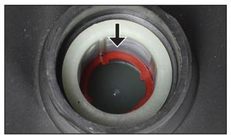
Figure 21 – Reinstalling the Fuel Strainer
