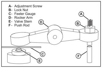
Figure 30 – Adjusting the Valve Clearance
