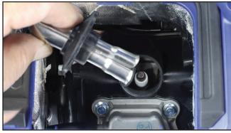
Figure 23 – Removing the Spark Plug Boot
