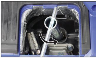
Figure 24 – Removing the Spark Plug
