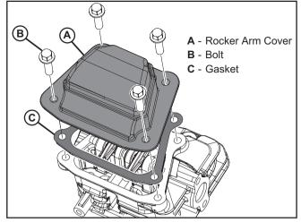
Figure 29 – Removing the Rocker Arm Cover
