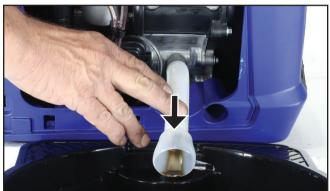
Figure 17 – Draining the Engine Oil
