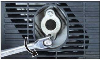
Figure 26 - Removing the Spark Arrestor Clamp
