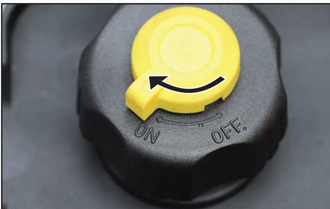
Figure 6 – Fuel Cap Vent in the ON Position
