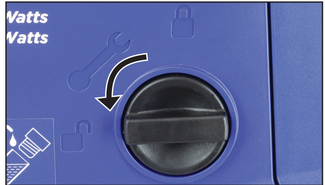
Figure 12 - RHS Maintenance Access Cover Lock in the Unlocked Position
