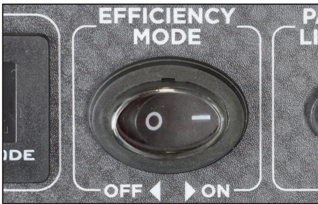
Figure 9 – ECO Throttle Switch in the ON Position
