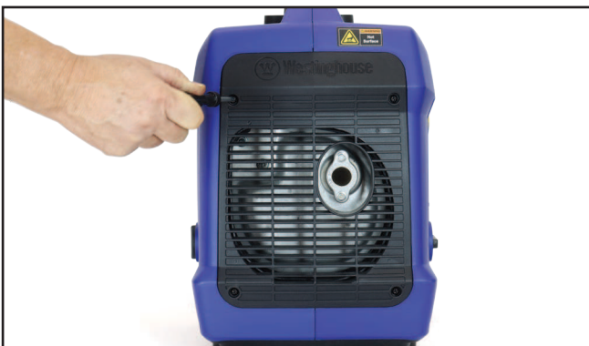
Figure 32 – Removing the Muffler Access Cover
