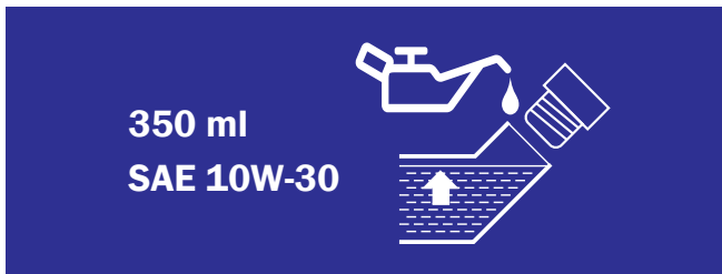
Figure 15 – Checking Oil Level
