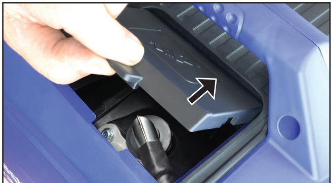
Figure 22 – Removing the Spark Plug Access Cover
