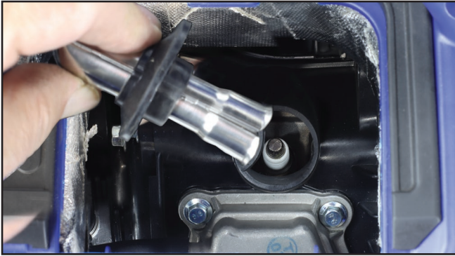
Figure 23 – Removing the Spark Plug Boot
