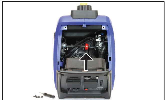
Figure 28 – Replacing the Fuel Filter
