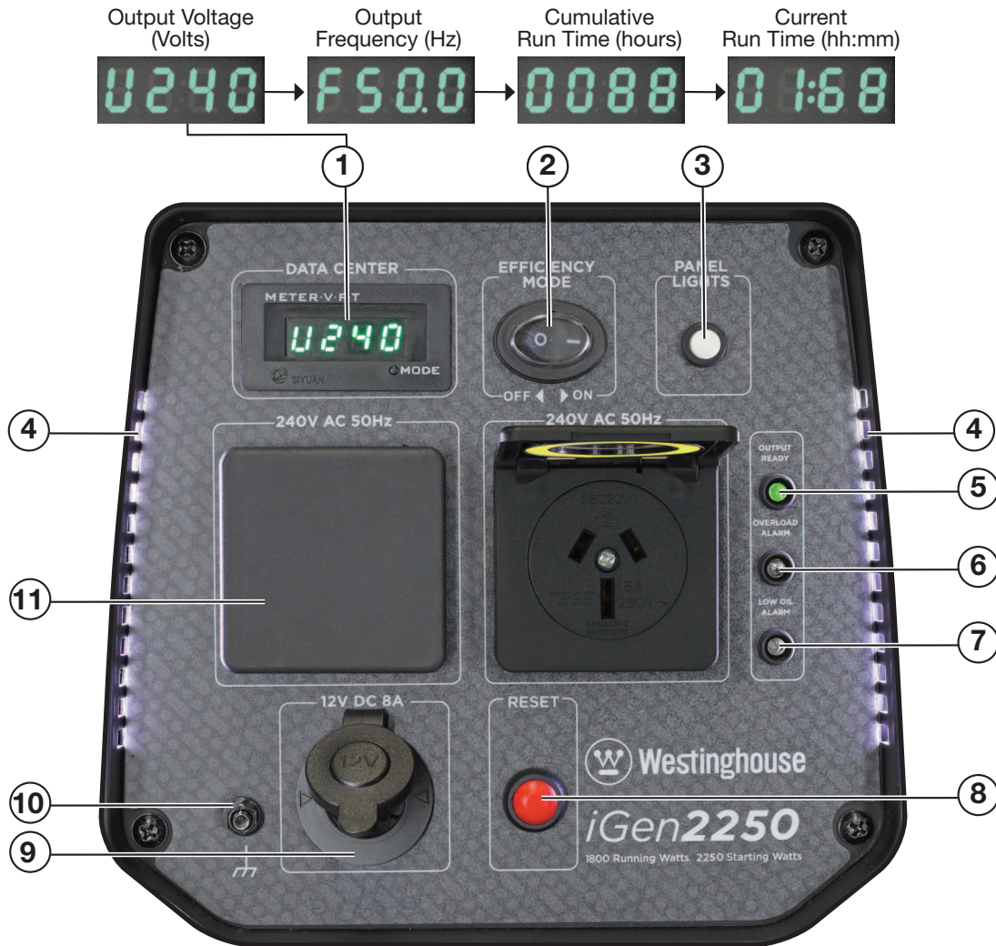
Figure 4 - iGen2250 Control Panel Features
