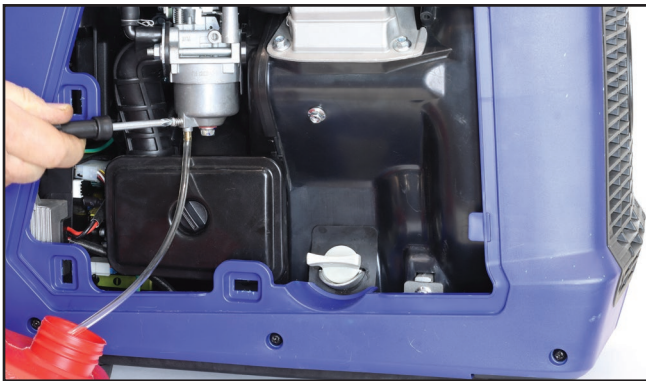
Figure 34 – Draining the Carburettor
