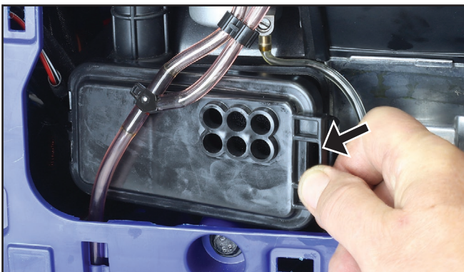
Figure 18 - Removing the Air Filter Cover
