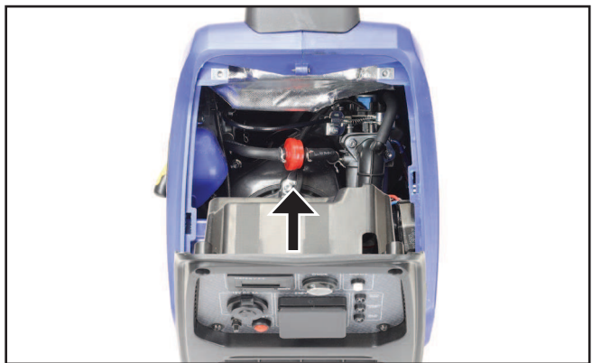
Figure 28 – Replacing the Fuel Filter
