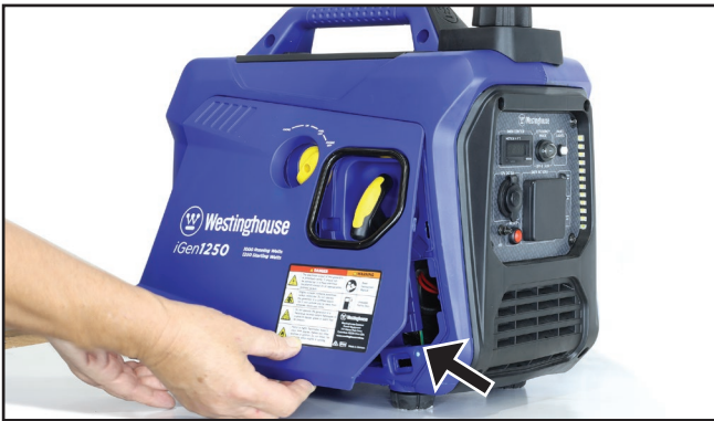
Figure 31 – Removing the LHS Maintenance Access Cover
