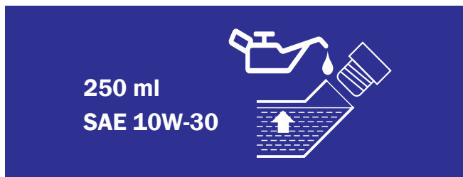
Figure 15 – Checking Oil Level
