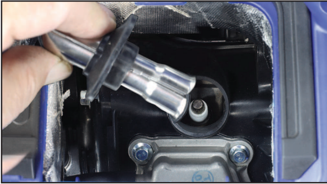
Figure 23 – Removing the Spark Plug Boot
