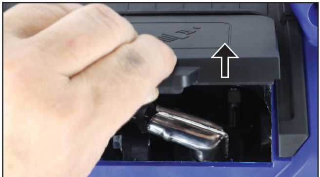
Figure 22 – Removing the Spark Plug Access Cover
