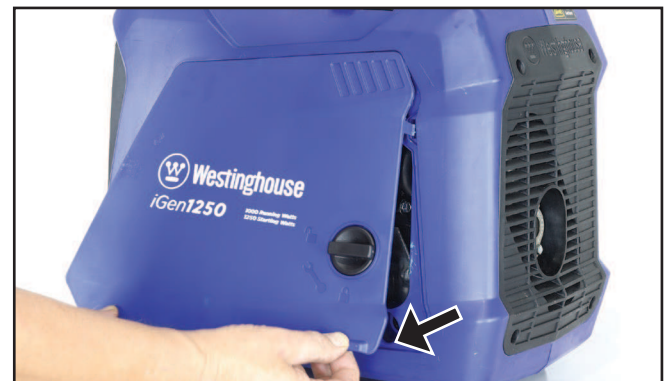
Figure 13 - Removing the RHS Maintenance Access Cover
