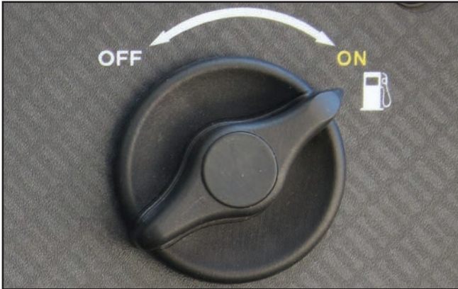
Figure 18 – Fuel Control Switch in the ON Position
