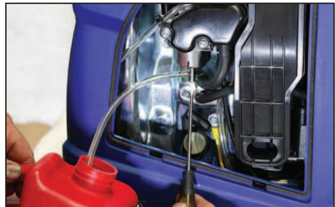
Figure 51 – iGen1200 Draining the Carburettor
