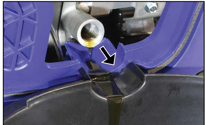
Figure 32 – Draining the Engine Oil
