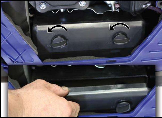
Figure 36 - iGen4500 Removing the Air Filter Cover
