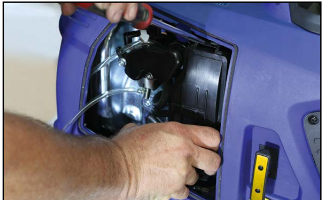
Figure 34 - iGen1200 Removing the Air Filter Cover
