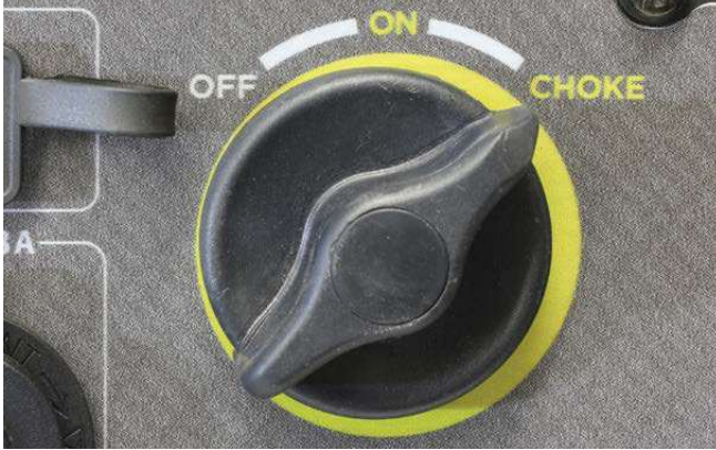
Figure 18 – Fuel and Choke Control Switch in the CHOKE Position
