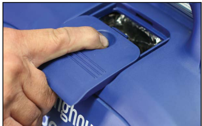
Figure 41 - iGen2200 & 2500 Removing the Spark Plug Access Cover
