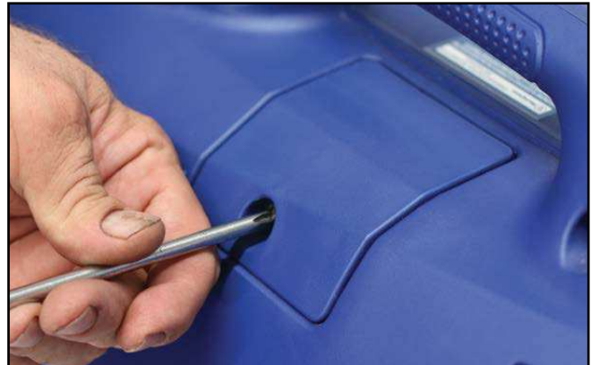
Figure 40 - iGen1200 Removing the Spark Plug Access Cover
