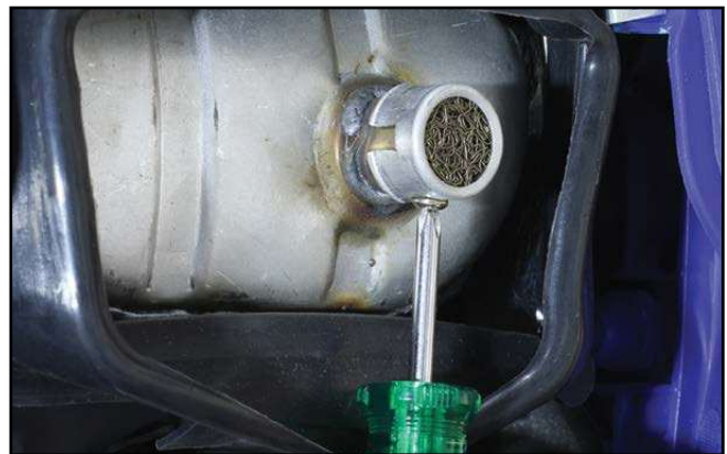
Figure 48 - Removing the Spark Arrester Collar and Screen
