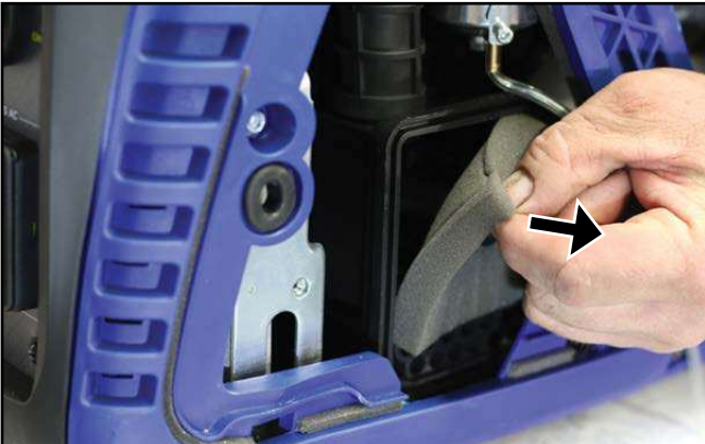
Figure 37 - Removing the Air Filter Element
