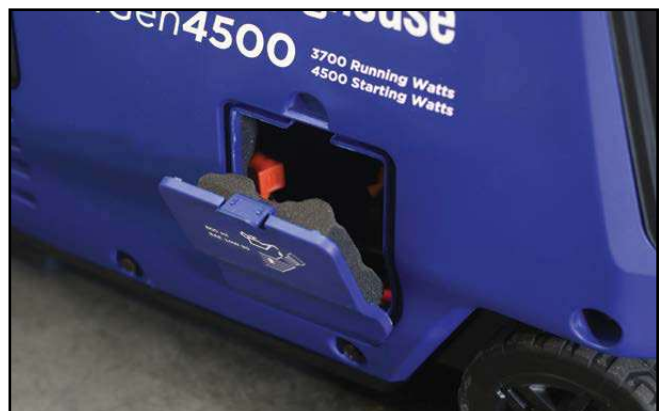
Figure 28 - iGen4500 Removing the Oil Access Cover
