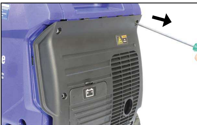
Figure 46 – iGen4500 Removing the Muffler Access Cover
