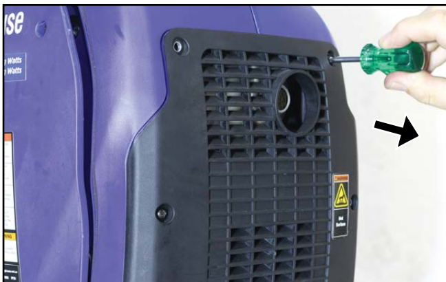
Figure 45 – iGen2200 & 2500 Removing the Muffler Access Cover
