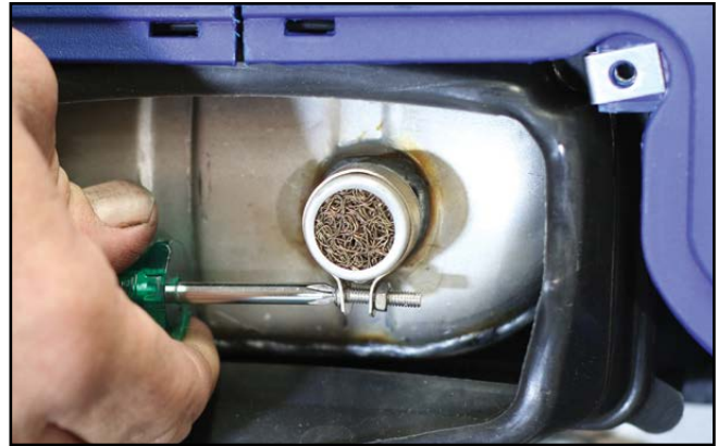
Figure 47 – Removing the Spark Arrester Band Clamp
