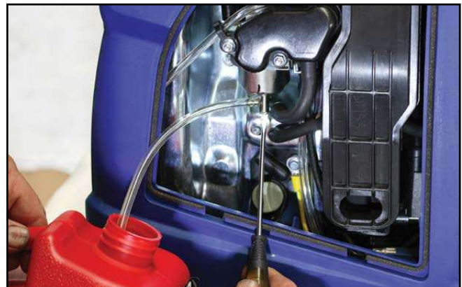
Figure 50 – iGen1200 Draining the Carburettor
