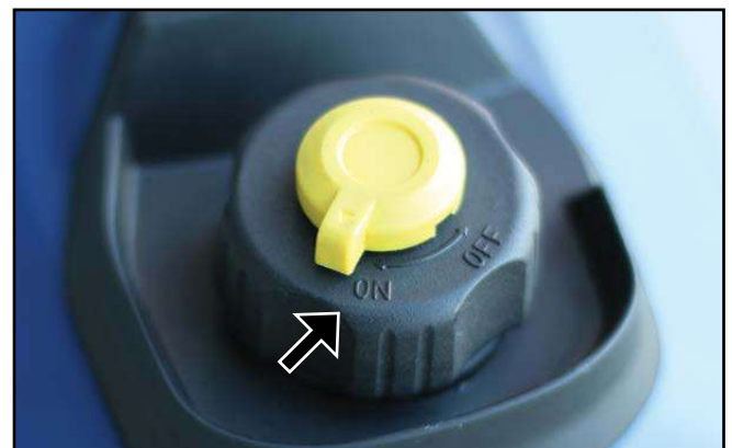
Figure 13 – Fuel Cap Vent in the ON Position
