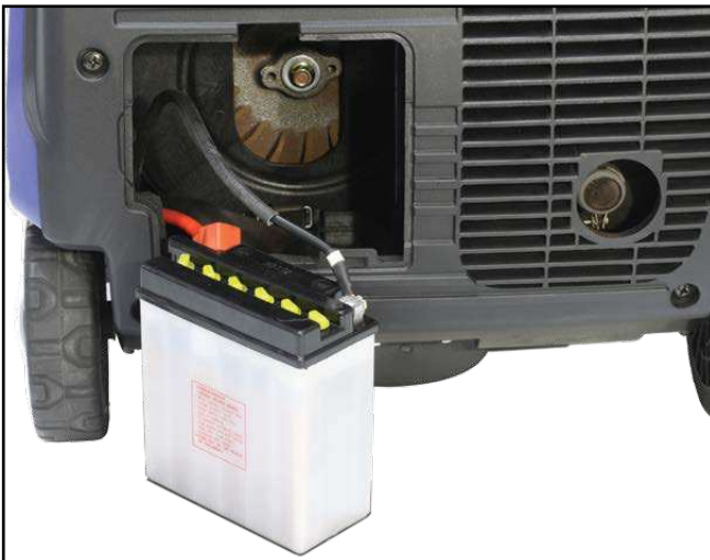
Figure 10 – Battery Removed from Generator for Connection
