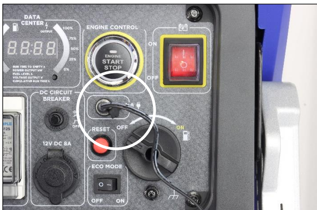
Figure 34 Connecting the Battery Charger to the Generator
