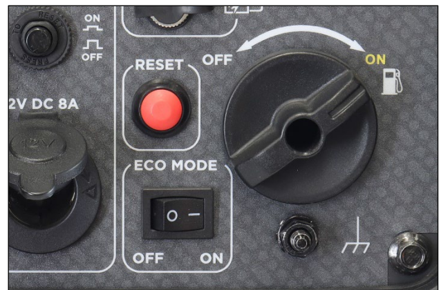
Figure 13 Fuel Control Switch in the ON Position
