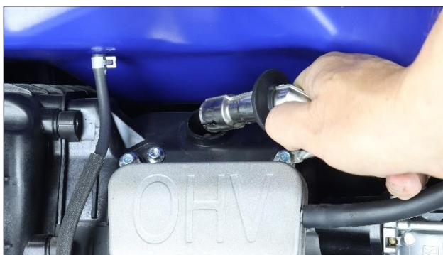
Figure 43 Remove the Spark Plug Boot
