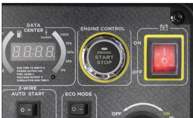
Figure 14 Battery Switch in the ON Position
