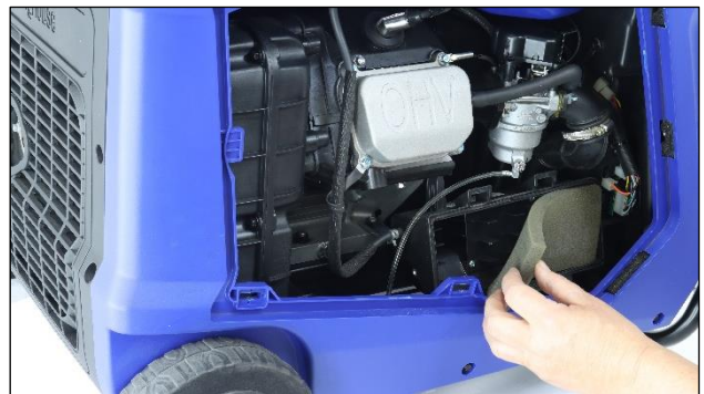
Figure 37 Remove the Air Filter Element
