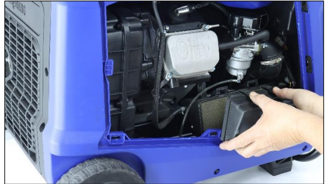
Figure 36 Remove the Air Filter Cover
