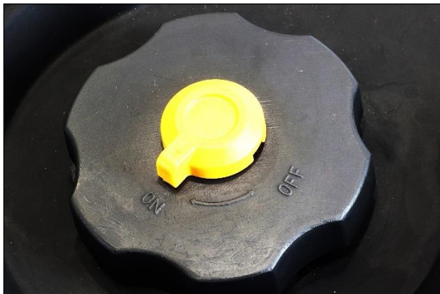
Figure 11 Fuel Cap Vent in the ON Position
