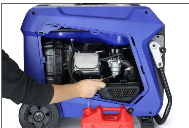
Figure 41 Drain the Carburettor
