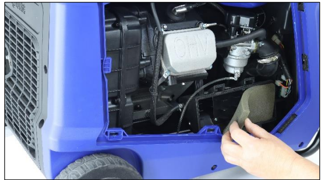
Figure 37 Remove the Air Filter Element
