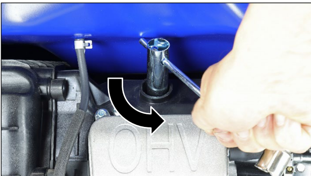
Figure 44 Remove the Spark Plug
