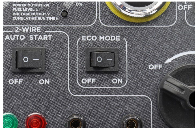
Figure 20 ECO Mode Switch in the ON Position
