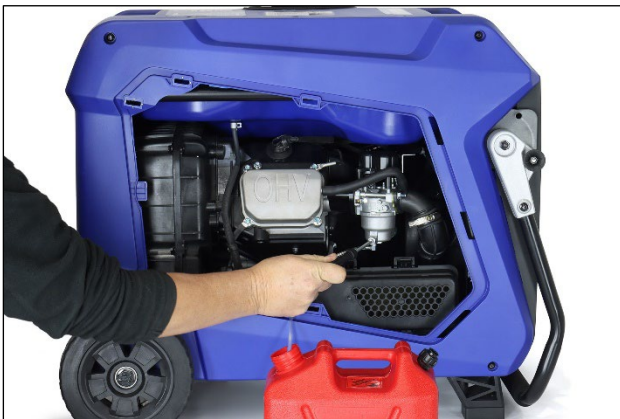
Figure 41 Drain the Carburettor
