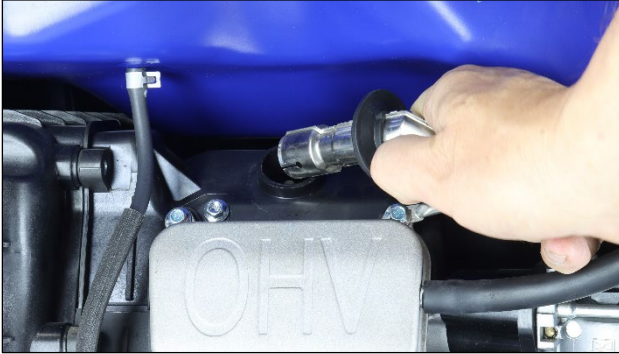
Figure 43 Remove the Spark Plug Boot
