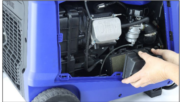
Figure 36 Remove the Air Filter Cover
