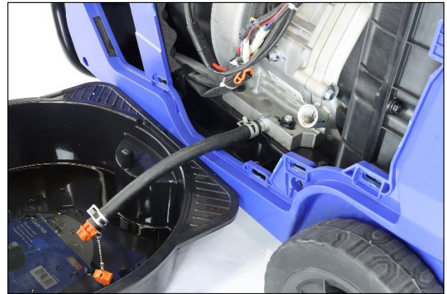
Figure 33 Draining the Engine Oil
