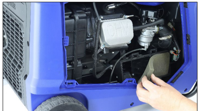
Figure 37 Remove the Air Filter Element
