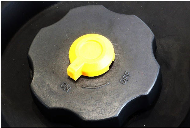
Figure 11 Fuel Cap Vent in the ON Position
