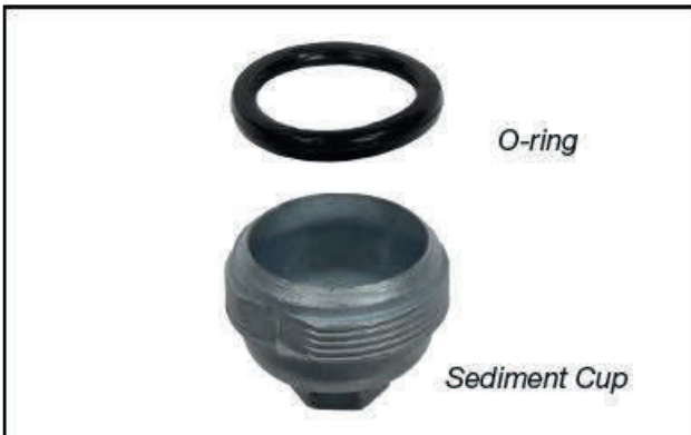
Figure 34 Fuel Sediment Cup and O-ring
