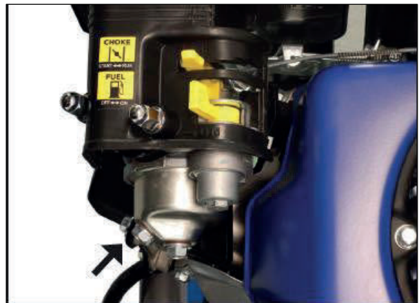
Figure 36 Remove the Carburettor Drain Screw
