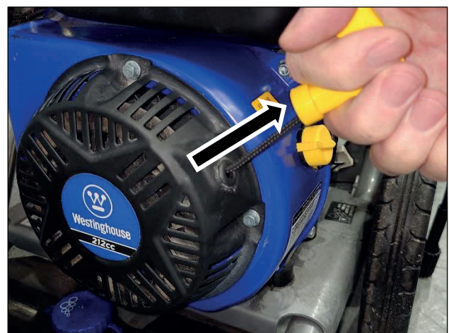
Figure 20 Recoil Starter Handle Operation
