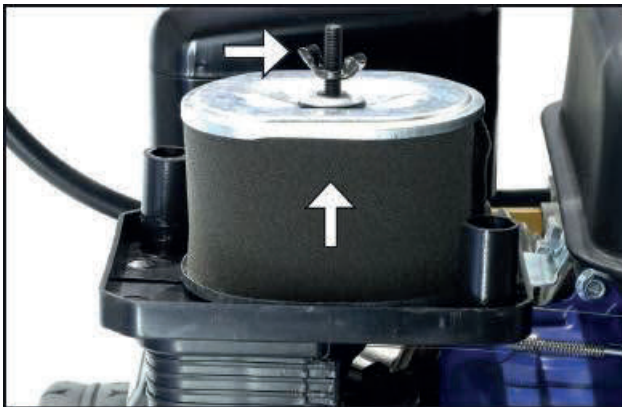
Figure 29 Remove the Air Filter Elements
