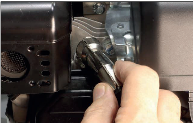
Figure 37 Removal of Spark Plug Boot
