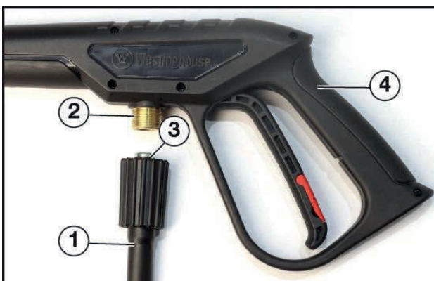
Figure 10 Connecting Pressure Hose to Spray Gun
