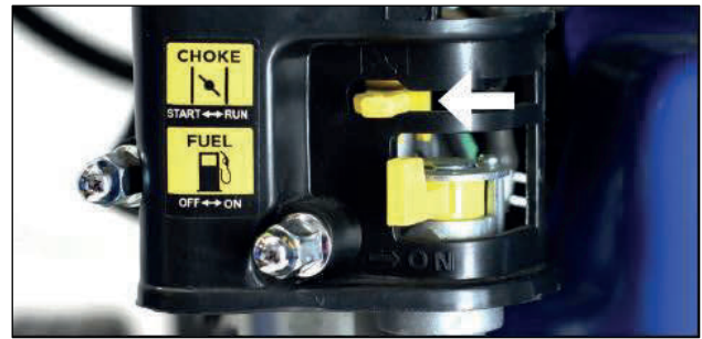
Figure 18 Choke Lever in the START Position
