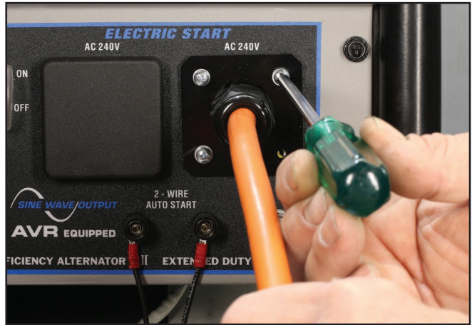
Figure S9 – Affixing the Gland Plate to the Control Panel
