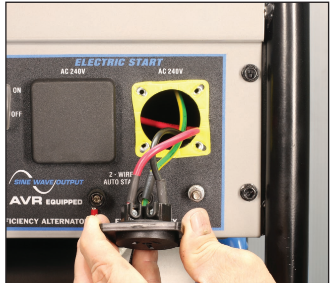
Figure S5 – Withdrawing the 240-Volt AC Socket
