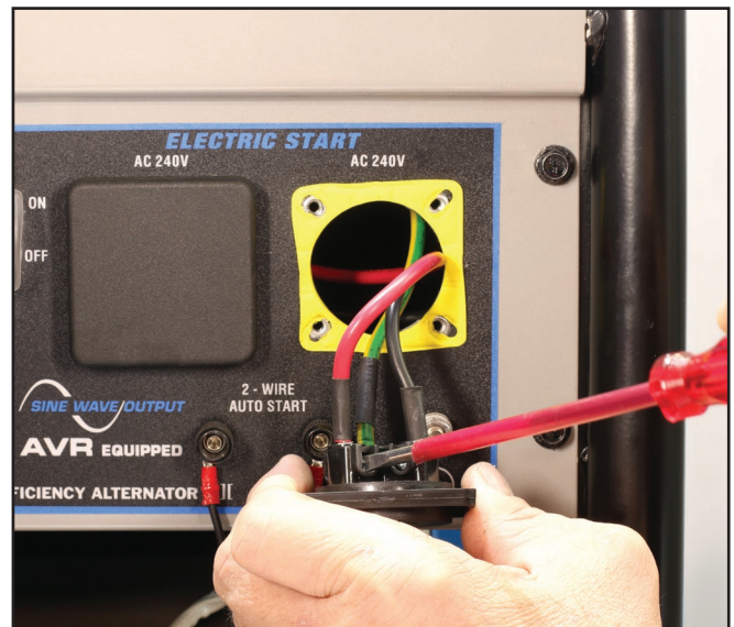
Figure S6 – Disconnecting the 240-Volt AC Socket
