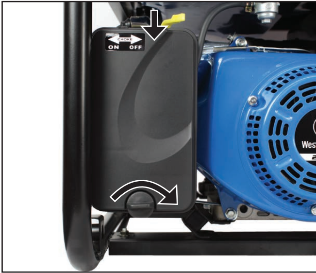
Figure 37 – Installation of Air Filter Cover
