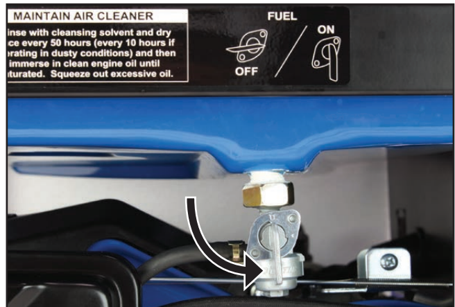
Figure 22 – Fuel Shutoff Valve in the ON Position
