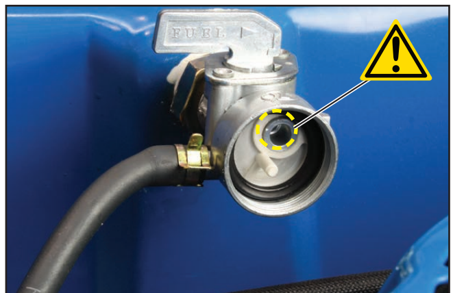
Figure 46 – Re-installing Fuel Sediment Cup Filter
