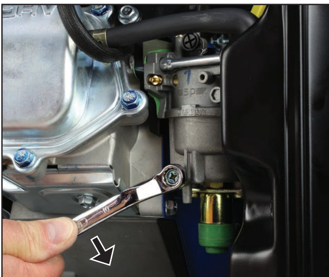
Figure 57 – Removing the Carburettor Drain Screw (WHXC5000, WHXC7000, WHXC8500E, WHXC8500E-PRO & WHXC8500E-AS)
