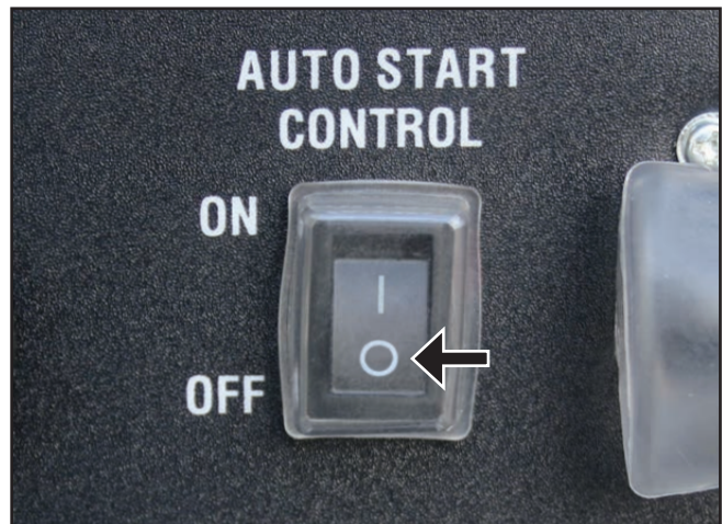
Figure 15 – Auto Start Control Switch in the OFF Position
