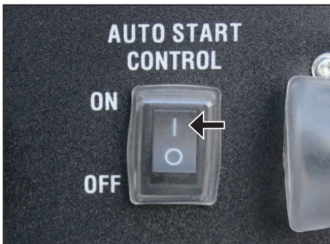
Figure 26 – Auto Start Control Switch in the ON Position
