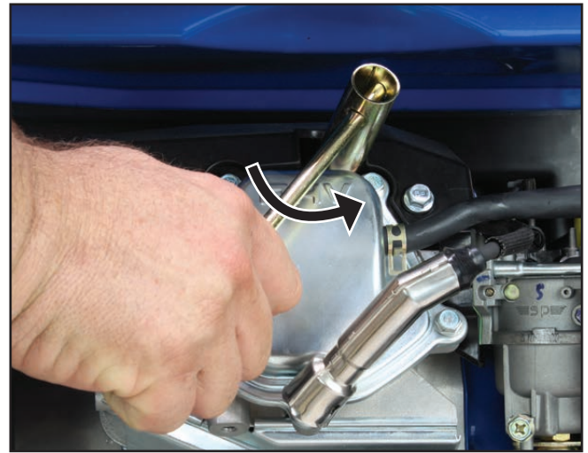
Figure 48 – Removing Spark Plug
