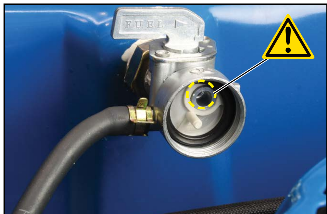
Figure 46 – Re-installing Fuel Sediment Cup Filter
