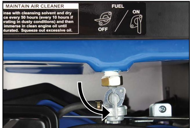
Figure 22 – Fuel Shutoff Valve in the ON Position
