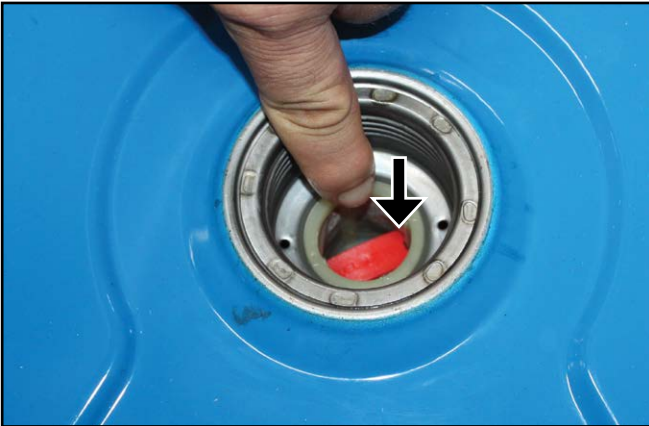
Figure 43 – Re-installing Fuel Strainer
