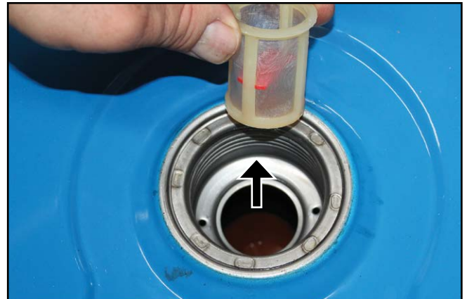
Figure 42 – Removing Fuel Strainer.
