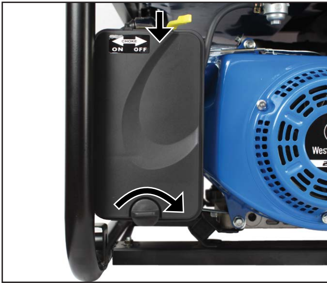
Figure 37 – Installation of Air Filter Cover
