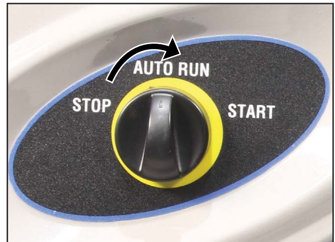
Figure 19 - Engine Control Switch in the AUTO RUN Position
