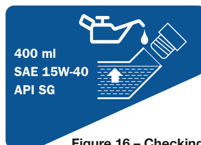
Figure 16 – Checking Oil Level
