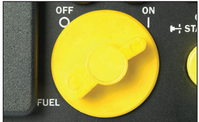
Figure 8 – Fuel Control Switch in the ON Position
