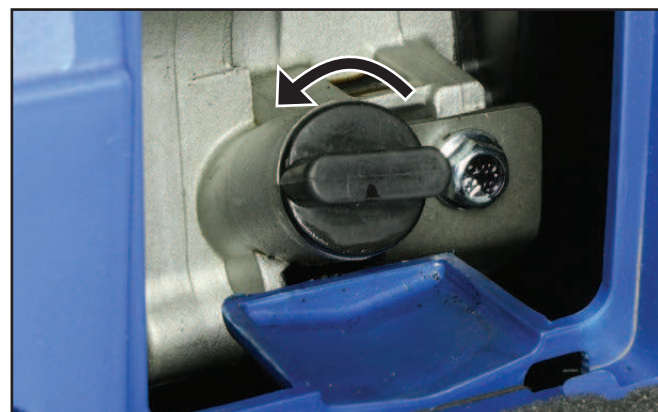
Figure 15 – Removing the Oil Fill Plug
