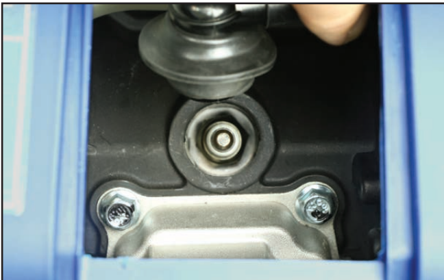
Figure 25 – Removing the Spark Plug Boot
