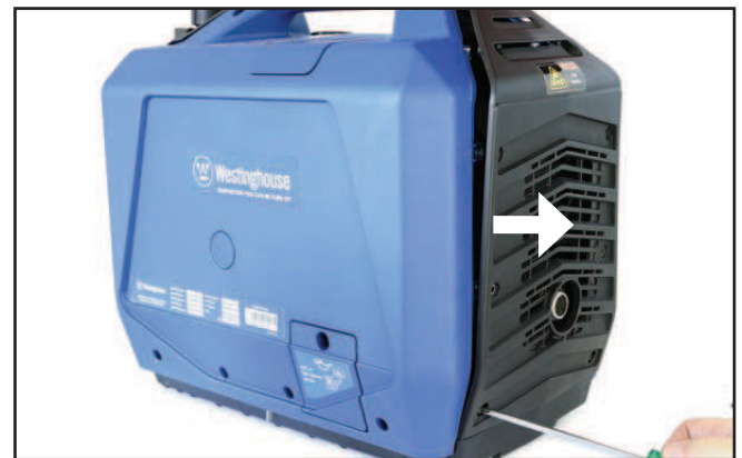
Figure 28 – Removing the Muffler Access Cover
