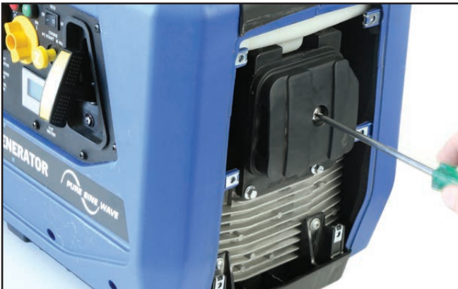
Figure 20 – Removing the Air Filter Cover
