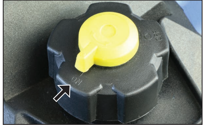
Figure 7 – Fuel Cap Vent in the ON Position
